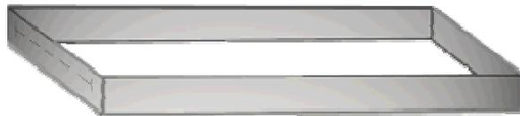
Use 1/4 inch aluminium angle moulding for the riffles. Drill through the angle and plastic of the tray to position the riffles. Cut down one end of the tray to the level of the discharge riffle.
